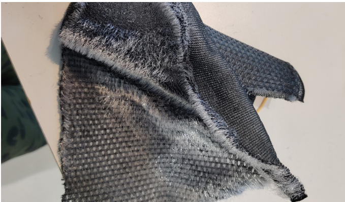
Figure 9 Plastic strings inside spacer fabric
